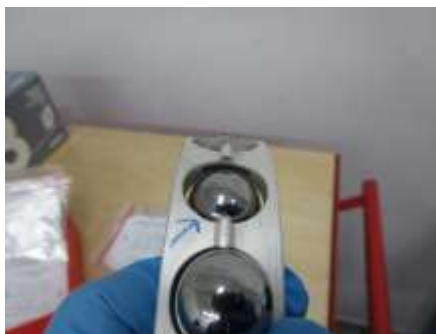
No. 1 Brg. - Flaking at cage
