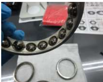
No.3 Brg. -Flaking of inner diameter of cage.
