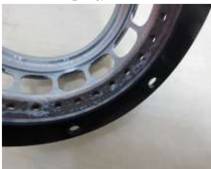
No.4 Brg: Corrosion on more than 30% of Area 1
