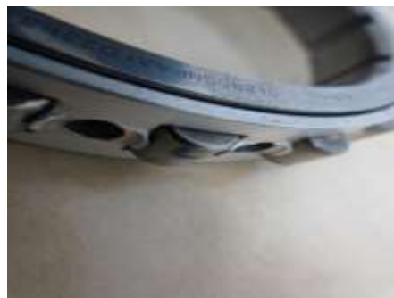
No.2.5 Brg. Dents on Roller Elements
