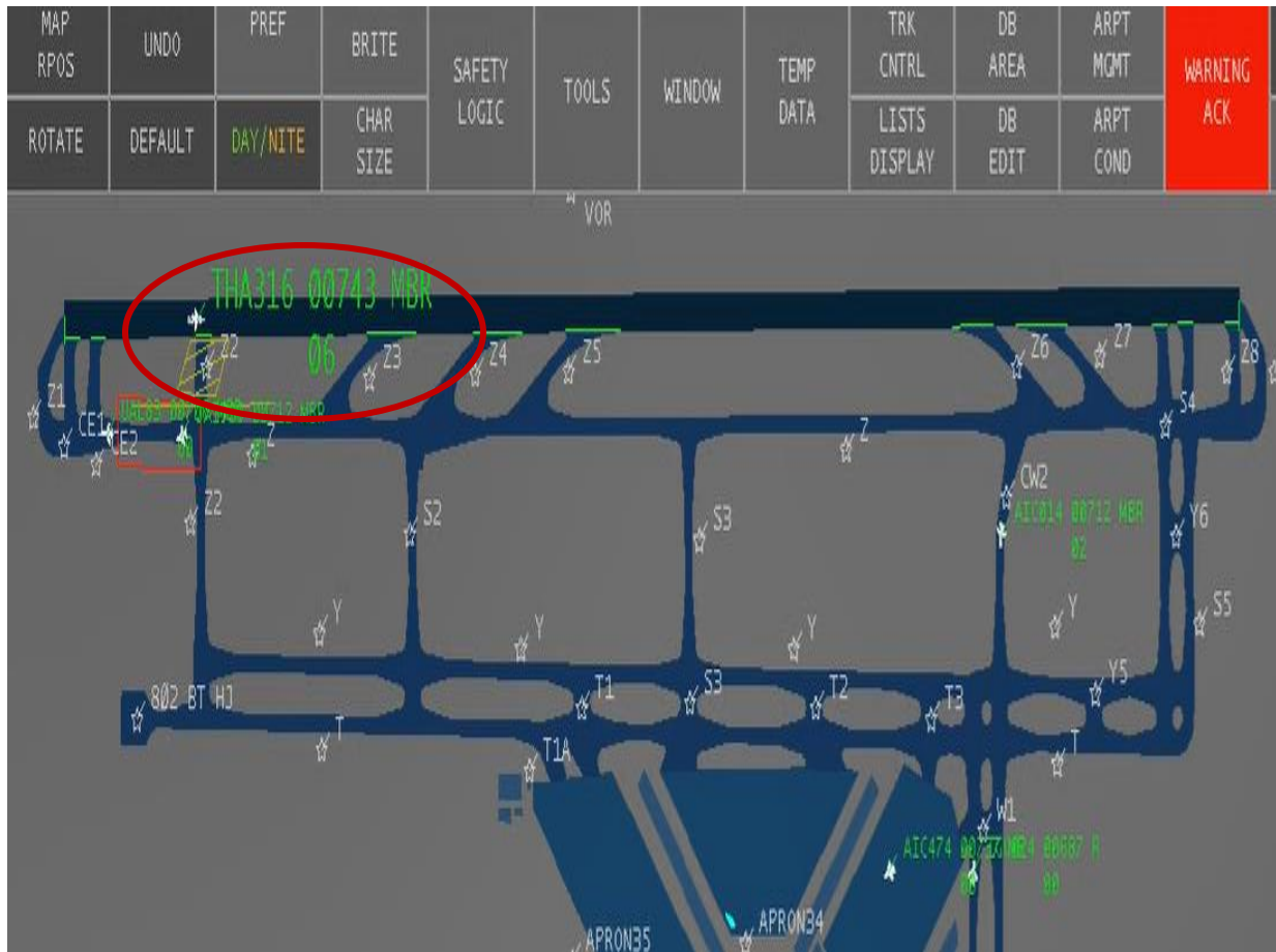
Figure 7: THA316 rolling RWY29 position abeam Twy Z2 at time 18:24:02
